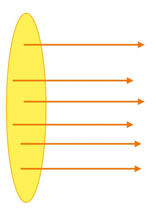
We have a media that absorb the photon  $\exp(-c_0 x)$ , Beer's Law, where *c* is a constant of the media and *x* is the travelled distance.
